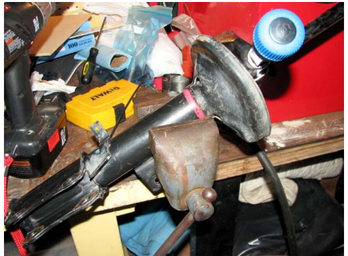
Figure 4 Secure the strut in a vice at approximately the angle shown to prevent oil from pouring out while you complete your cut.
