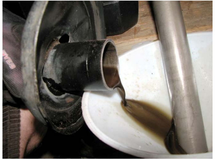
Figure 6 Complete the cut. Remove the inner tube, piston, and piston rod assembly. Drain the strut tube. The shock oil can be recycled with your motor oil. Using a file, clean up the inside of the cut to make sure it's at least flush to the ID of the tube. You may also slightly bevel the edge to facilitate installation later.
