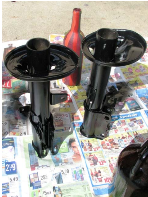
Figure 8 For extra style points at your next road race, scuff the paint with a Brillo pad or sand paper, clean thoroughly using a quality degreaser, and paint. I chose Rustoleum Appliance Epoxy paint for its scratch resistance qualities.
