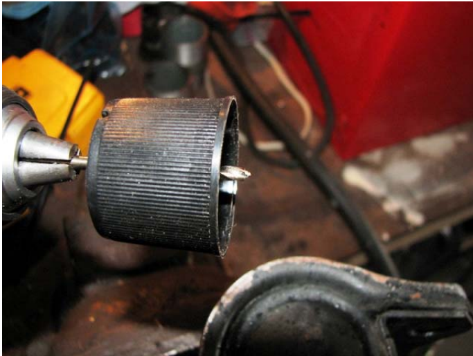
Figure 1 CAUTION: If struts are in good shape, gas/oil may vent. I suggest making a spray shield out of spray can lid.
