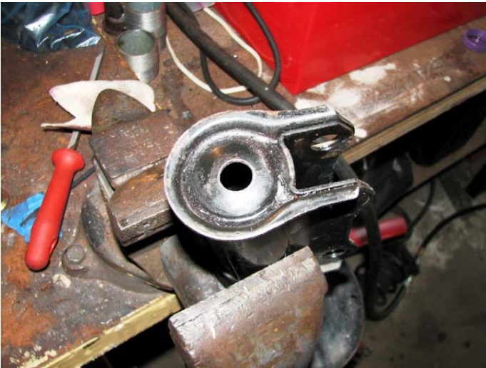
Figure 7 Turn the strut tube over and enlarge the hole in the base with a 14mm (or 9/16") drill bit as shown.
