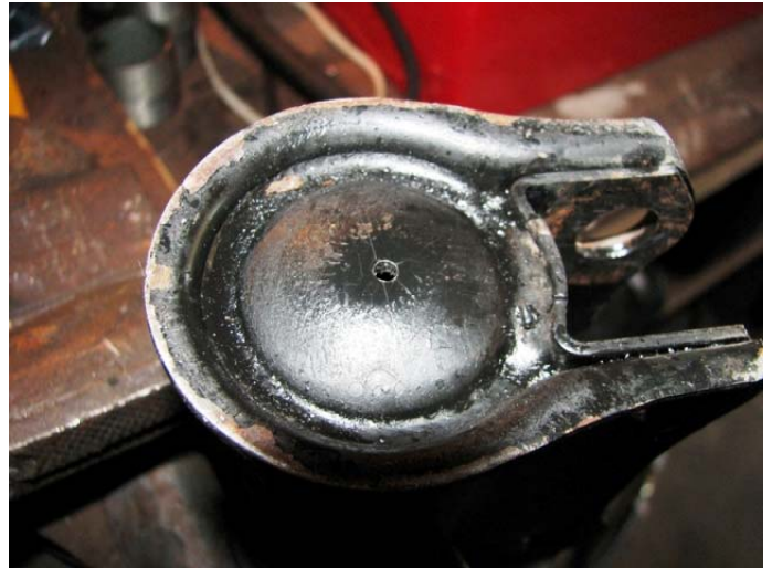
Figure 2 Make a small divot in the middle of the strut base with an awl or nail. Carefully drill through the base with a 3mm (or 1/8") drill bit.
